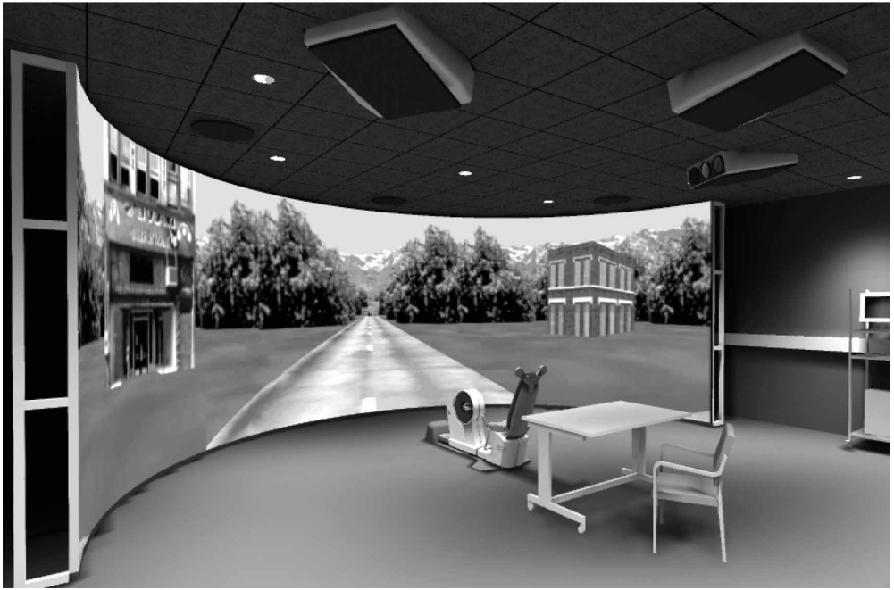
Figure 2. The virtual environment apparatus used in the experiment. The participants were placed on the training bike in front of the half-cylindrical screen.
