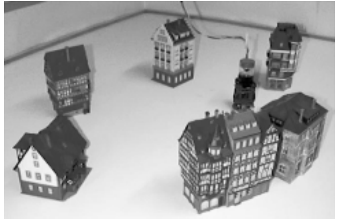
Fig. 4. Test arena ( 118 \times 102 cm) with toy houses, used in the homing experiments (see Sect. 5.1). The modified Khepera robot is depicted in the right half of the arena
