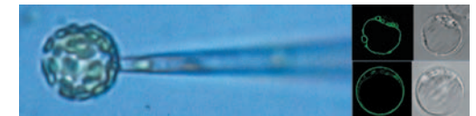
Fig. 4: Transformed plant protoplasts expressing GFP-tagged plasma membrane (lower inset) or tonoplast channels/ transporters (upper inset) are identified by their fluorescence. Transport in individual protoplasts or vacuoles is then analyzed by patch clamp.
