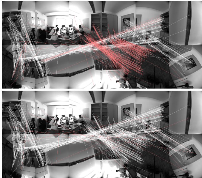
Fig. 9. Failing 2D orientation vs. nicely separating 3D orientation based match refinement. 2D histogram based (top, Section IV-A1) vs. 3D mean (bottom, Section IV-B1) strategy. White lines represent selected, red lines discarded features. Our 3D refinement discards false matches selectively in the entire omnidirectional image while the 2D refinement only succeeds for a compact region of viewing directions, discarding lots of inliers.
