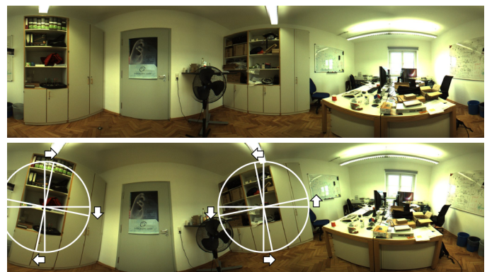
Fig. 2. Omnidirectional images with straight (top) and rolled (bottom) camera. Note how the image areas in the back facing part rotate inverse to the front, so there is no common 2D feature rotation.
