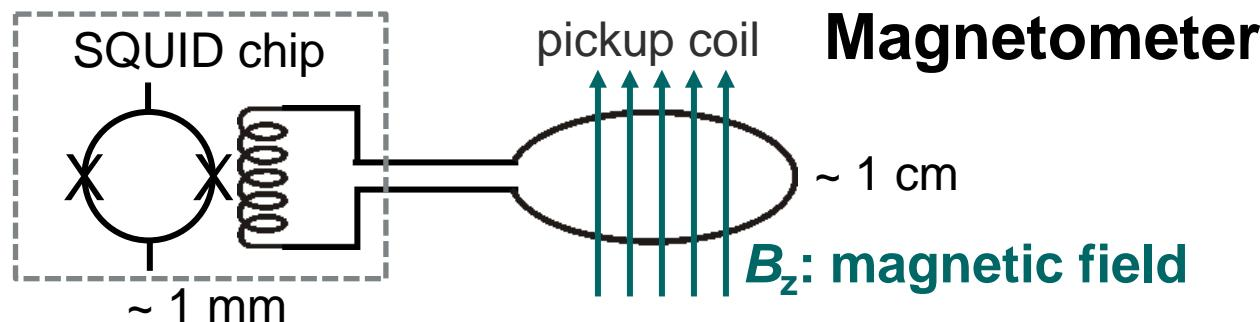
**field noise:**  $\Phi_n/A_{\text{eff}} = B_n \sim 1 \text{ fT} \cdot (\Delta f/\text{Hz})^{1/2}$
