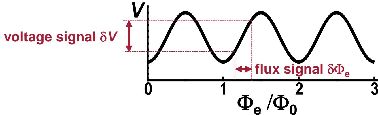
flux feedback electronics → linear voltage-to-flux response
