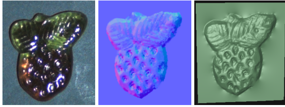
Figure 3: The photo of a jelly candy, exhibiting sub-surface scattering (left), a normal map acquired with the shape-from-specularity approach of Chen et al. [CGS06] (middle), and three-dimensional surface shape obtained by integrating the normal field. Image courtesy of Tongbo Chen, Michael Goesele and Hans-Peter Seidel.
