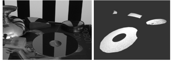
Figure 4: Shape reconstruction of specular objects using direct ray measurements. An input photograph with three curved and one planar specular object (left) and reconstruction result seen from a different view-point (right). The large object to the left has only been partially reconstructed due to missing pattern information. Image courtesy of Thomas Bonfort, Peter Sturm and Pau Gargallo [BSG06].
