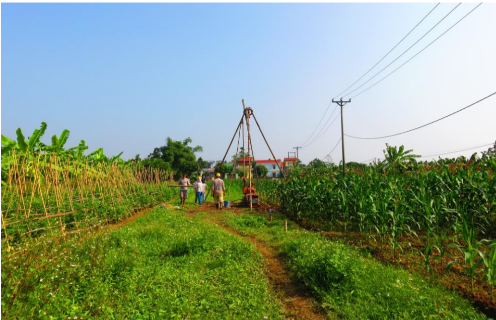
Drill cores were taken in 2018 in Van Phuc, Vietnam, for laboratory experiments investigating the origins of methane and arsenic in the groundwater. Photo: Andreas Kappler
