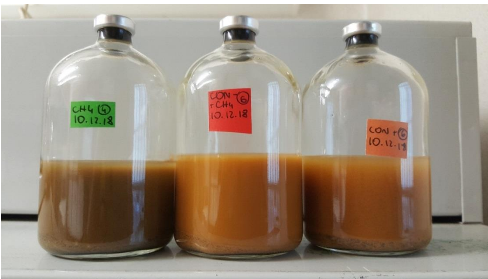
Sediment incubation experiment. Methane supplied to sediment triggers mediated microbial Fe(III) mineral reduction and dissolution, mobilizing arsenic – as seen by the changing color of the sediments from orange (right) to dark brown (left). Photo: Andreas Kappler
